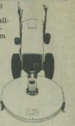
Gravelly 7.6 HP Convertible with 30" Rotary Mower Attachment
